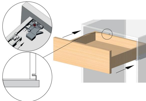
4. Adjust the front panel with plastic wheel on the handle, 0-2.5mm
