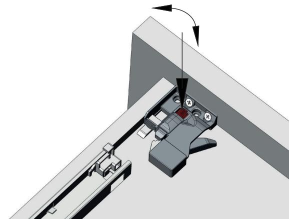
5. Push the handle lever to unlock the drawer, then pull out the drawer
