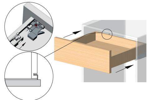
4. Adjust the front panel with plastic wheel on the handle, 0-2.5mm
