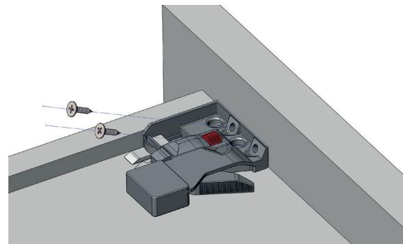
3. Install the drawer on the runners, slide hooks insert into the pre-drilled holes on the drawer back panel
